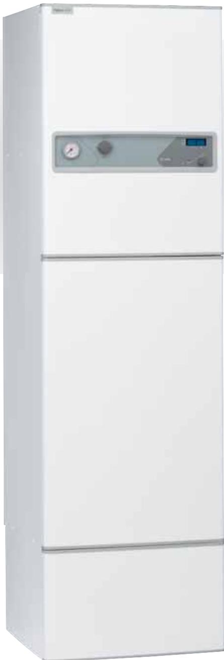
Mechanical ventilation system (central supply air) combined with a heat pump, which heats the domestic hot water and radiator water using exhaust air energy and preheats the fresh supply air.
